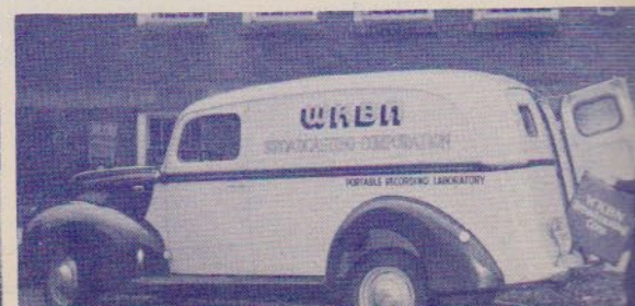
One of WKBN's portables. Complete equipment is carried by these vehicles for remote broadcasts--away from the studios. In effect, the car is a portable recording laboratory.
